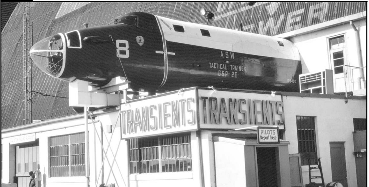
**ABOVE:** Remember the GSP-2E? This was the forward fuselage section of an SP-2E that had an engine fire on the ground at NAS Brunswick. It was trucked to NAS South Weymouth and mounted on top of the south lean-to on the side of Hangar One, wired up to simulation equipment in the ASW Training Department's spaces, and was used as a tactical trainer for many years. Photo by Richard Sullivan courtesy of Stephen Miller. Got something similar to share? If so, contact Marc J. Frattasio.
